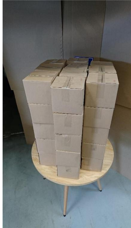
**Under the strain of close to 550 kg. the setup was gently pushed from side to side and back and forth for several minutes – not done in any scientific way.**
