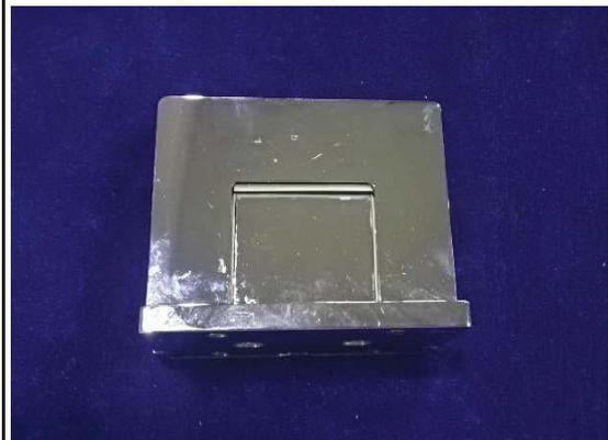
After 240 hours salt spray test
