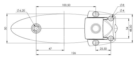
1 set consists of a male & female part made of PA6 material. Fixation by means of 4 wood screws, a zamak screw-in bushing and a fifteen screw.
