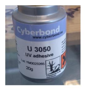
The hinge is glued onto a 12 mm. glass plate – picture below shows the result. The curing of the glue has been done by an appropriate UV light – wave length nm 380
