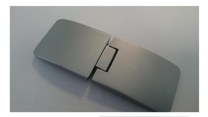
Dents / marks came from removing the hinge off the glass sheet. (done by hammer)
