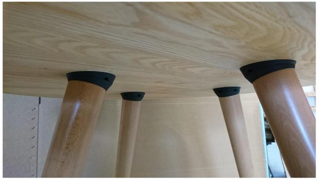
**Conclusion:** We put a strain on the 4 brackets of 547,80kg for a period of more than 60 hours.
