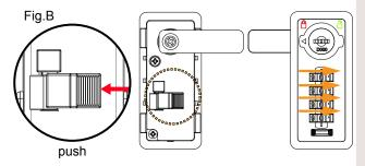
Push back the Decode Lever to its original place.
