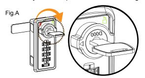
2. To retrieve the forgotten combination, push the Auxiliary Button to the left then it will stop the Decode Lever.
