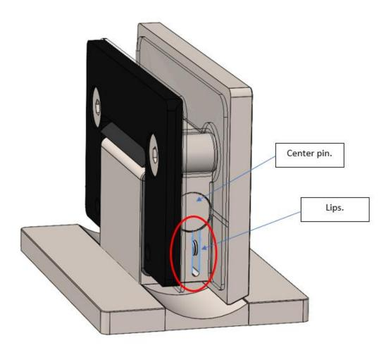
Normally, when loosening the small screws, these lip areas lose their grip and hold. But sometimes the areas keep the hold. This means the indicated area (on both sides of the hinge) needs to be spread apart for the center pin to rotate freely.
