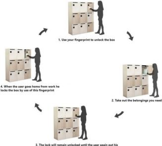
The lock will remain unlocked until the user aga finger to the fingerprint panel
