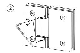
Tighten the set screws to fix the hinge to the desired angle
