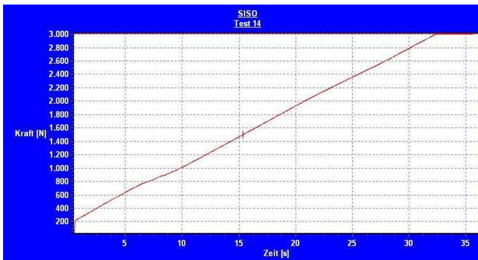
Fig. 20: static load test - for example model „OVAL-s“ 22.10.220-9
