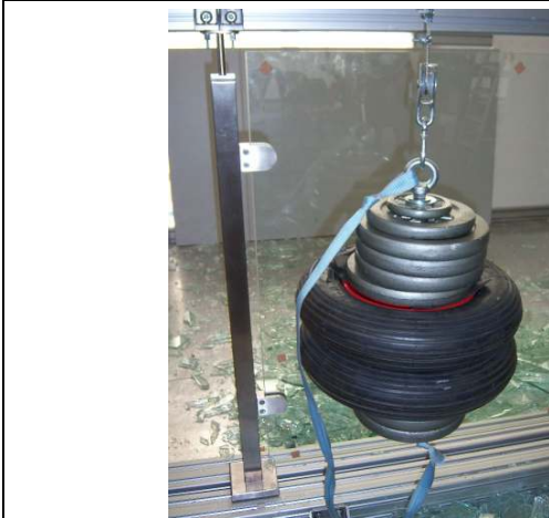
Fig. 15: pendulum test, 265 mm from one short edge (on the left side of the glass pane)
