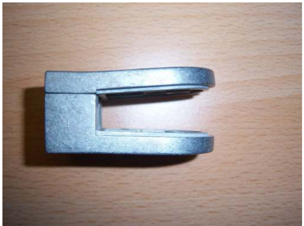
Fig. 8: Model OVAL-S, # 22.10.210-8, bended after static load
