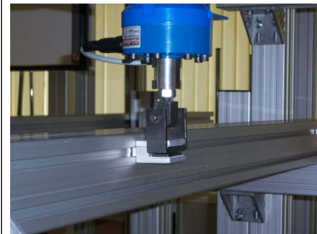
Fig. 17: static load test with glass clamp model „SQUARE“
