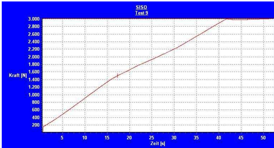
Fig. 19: static load test - for example glass clamp model „OVAL-L“ 22.10.220-8
