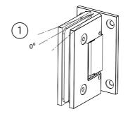
Adjust the glass door upon installation to the desired angle
