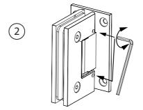
Tighten the set screws to fix the hinge to the desired angle
